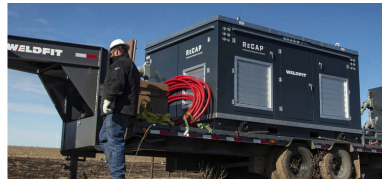
Equipment used to transfer methane captured from isolated pipeline sections to adjacent pressurized systems
